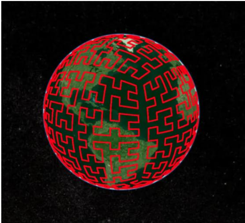
The S2 Hilbert curve on the WGS84 ellipsoid.
