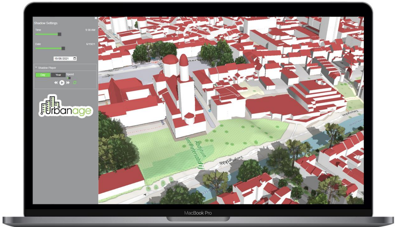
Figure 12: visualisation of shadow projection using terrain data, LOD-2 building information and tree data in the city of Ghent, Flanders.
