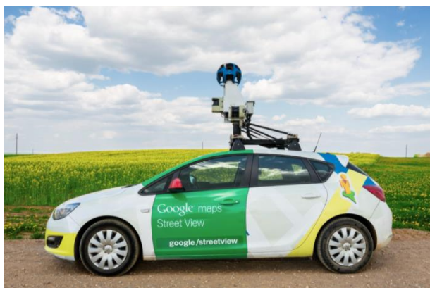
Figure 2 Google Street View car with camera mounted on top
